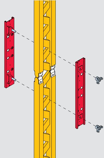
Horizontal extensions take place in a straight line; one extension splice is to be mounted per girder joint.
