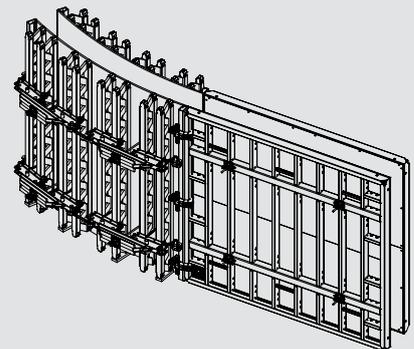
Straight outgoing walls can also be easily realized. For normal wall thicknesses, a 90 cm wide frame panel is used for this purpose on the outer side of the formwork; on the inner side, two articulated corners or two internal corners are connected.
